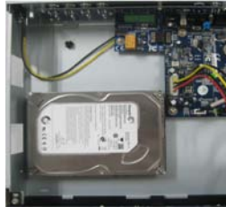
Fig 1.1 Connect HDD
